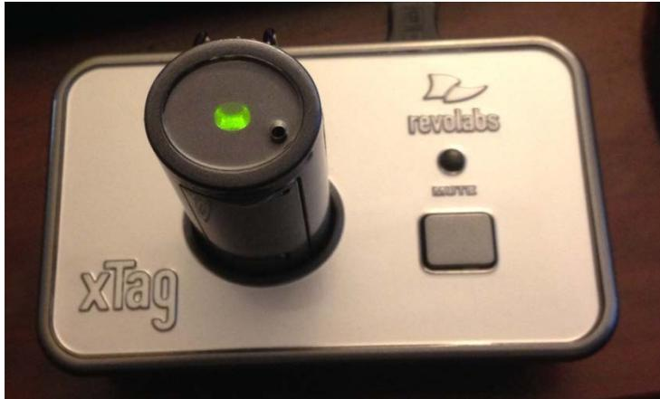
The *Revolabs xTag* wireless microphone operates after its USB plug has been plugged into a USB port on the computer. The computer will advise that the device is installing, and that it is then ready to use.
